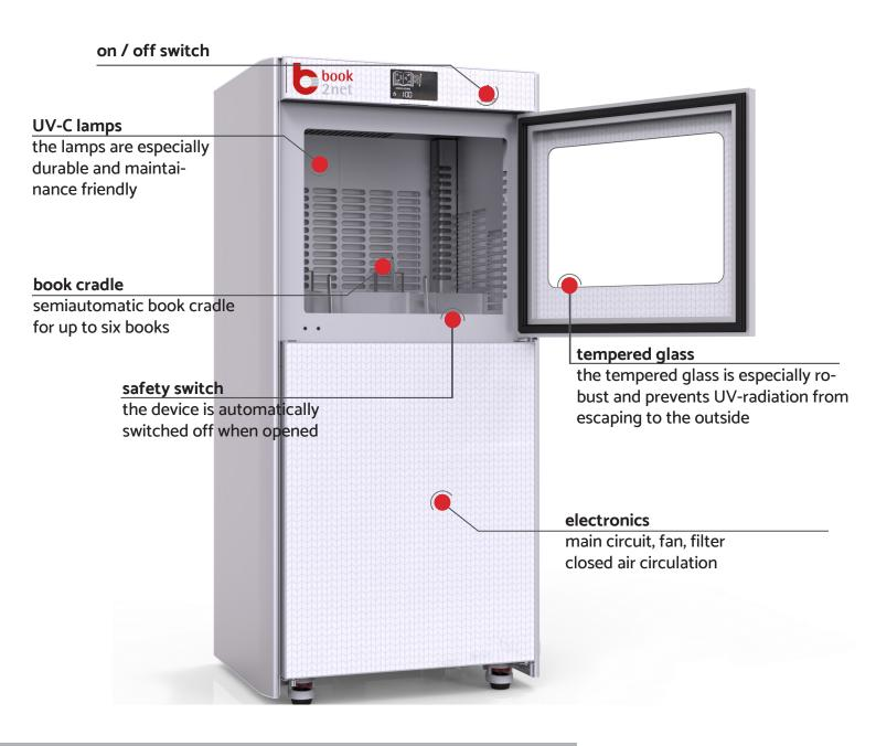
Size: 690(W)590(D)1420(H)mm Housing: Aluminum and steel Door: Aluminum and tempered glass (3.2mm) Connection values: 110v Energy consumption: 2.5watt Desinfection time: 30 seconds
